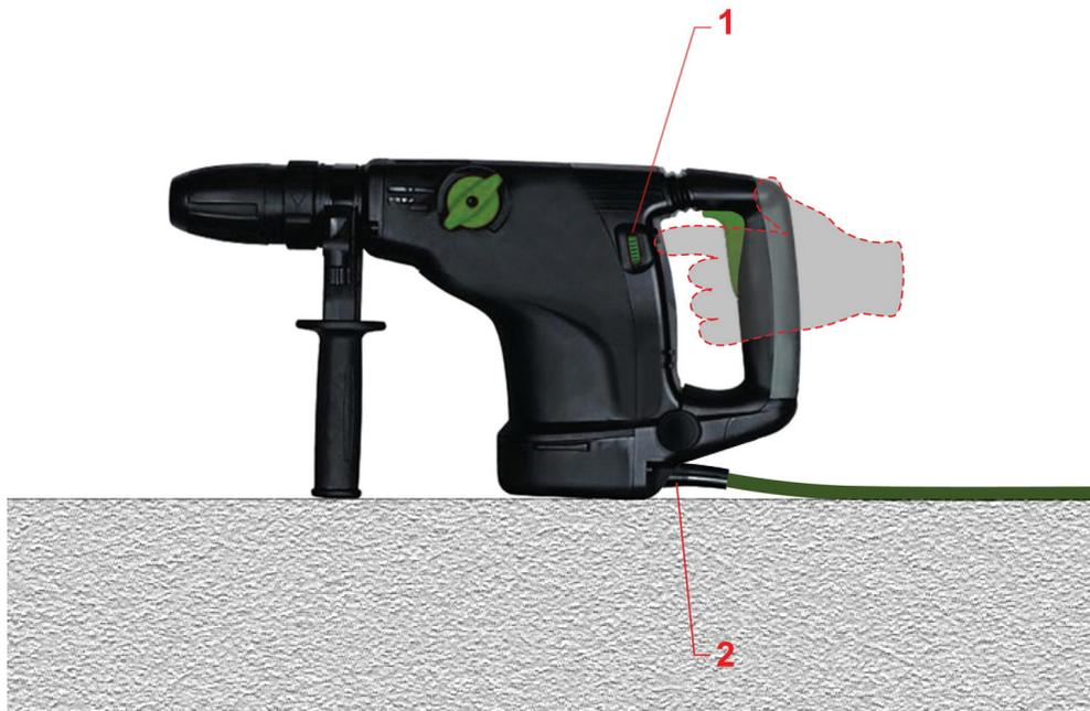
**Figure 7. The ergonomic position of the power cord and switch for speed control.**
