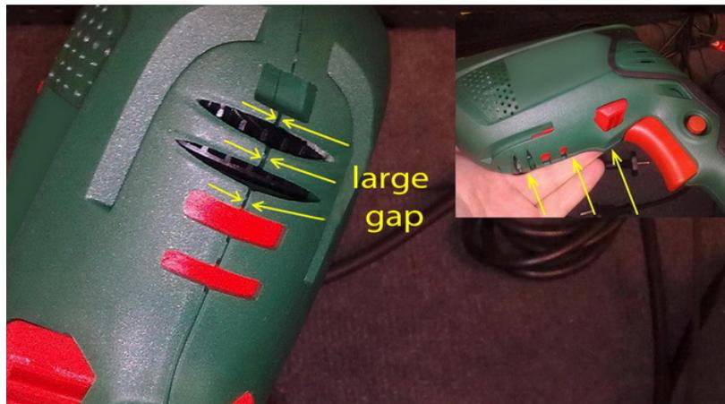
**Figure 2. Marked details show imprecision in assembling.**
