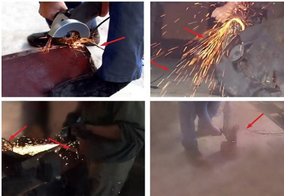
**Figure 3. Poor visibility during operation can lead to damage of the power cord.**
